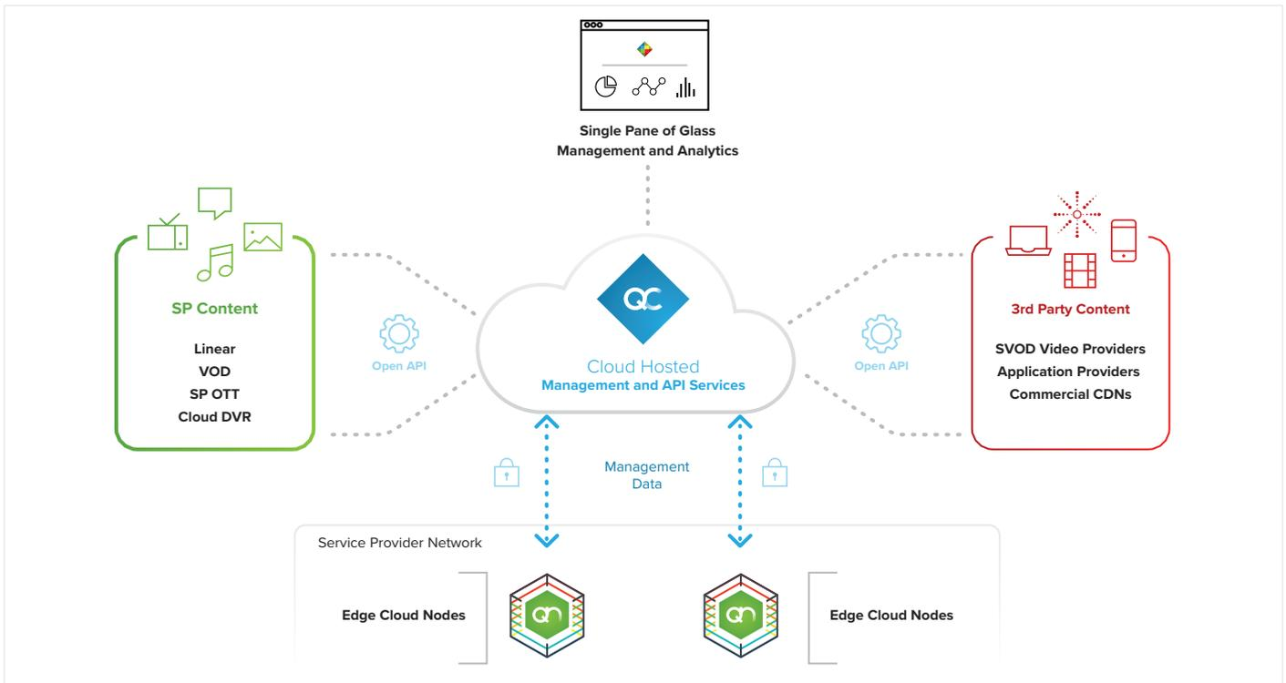
Figure 1. The Qwilt CDN features cloud-based QC control plane and QN edge delivery software.<sup>4</sup>
